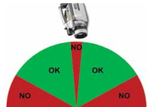
Viewing angle recommended (green) and to be avoided (red) during thermographic inspections.
